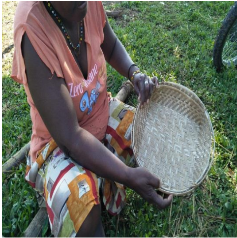
5. Process of bending the nito/darumaka/rattan upwards from the bottom of the basket
